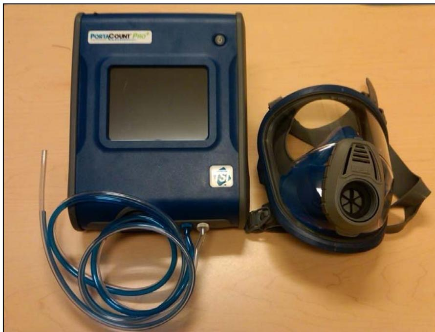
**Figure 12. The PortaCount Pro quantitative respirator fit testing machine. The blue tube takes in ambient air, while the clear tube takes in air from the inside of the respirator. The machine amplifies airborne particles using isopropyl alcohol and counts them in an internal chamber.**
